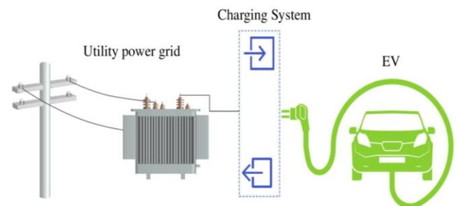
**Figure. 1** Schematic of the bidirectional charging system of V2G
