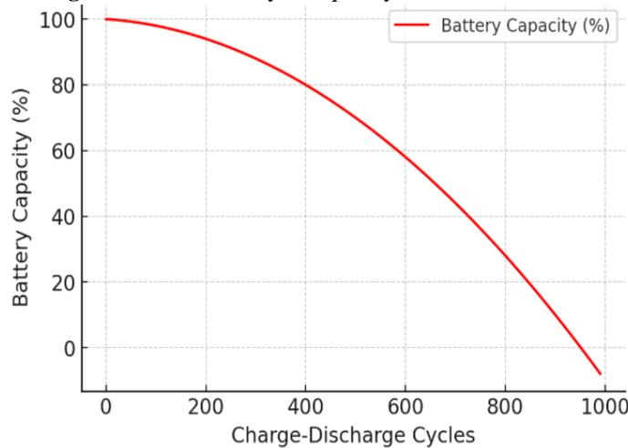
**Figure. 4** Battery Degradation Over Charge Cycle
