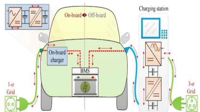
**Figure.2.** A simplified structure of single phase (on-board) and three-phase (off-board) bidirectional EV charging.
