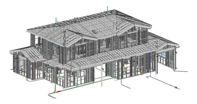
Below Image shows the Detailed over view of Floor panels for Light gauge steel along with all MEPF Services the way all of them managed well
