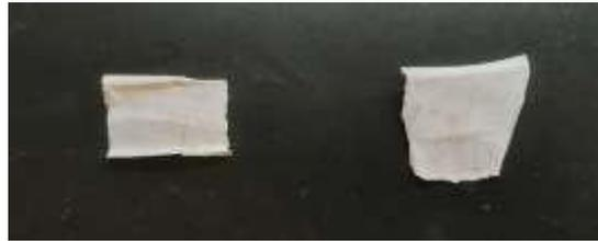
Fig 3.5 Comparative Corrosion Testing Of Normal And Nanoparticle Incorporated Paints On Metal Surfaces
