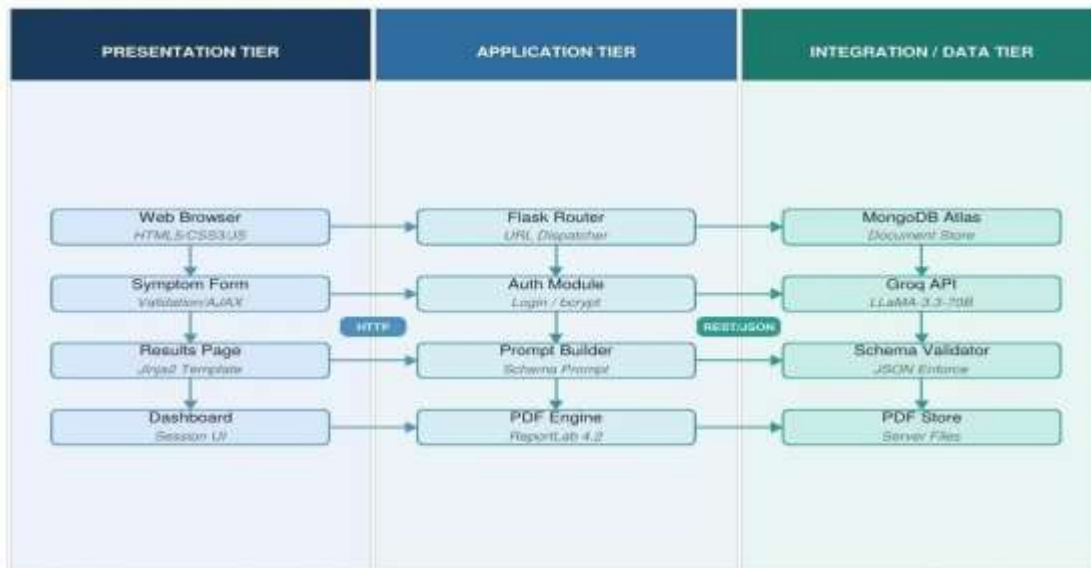
Figure 1: BDSAS Three-Tier System Architecture Diagram
