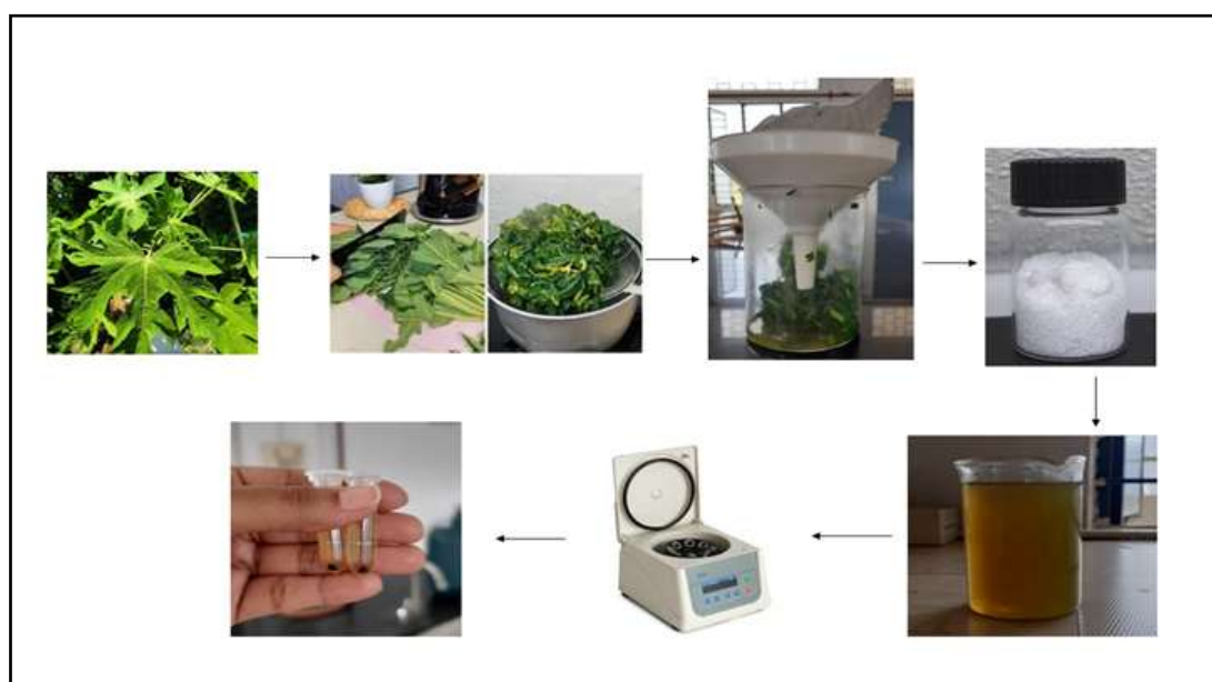
Figure 1. Steps involved in extraction of silver nanoparticles from C. papaya leaf extract.
