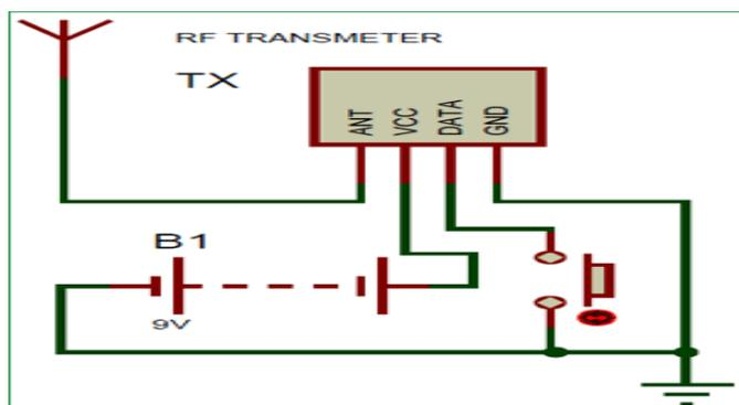
Fig -2 RF remote circuit
