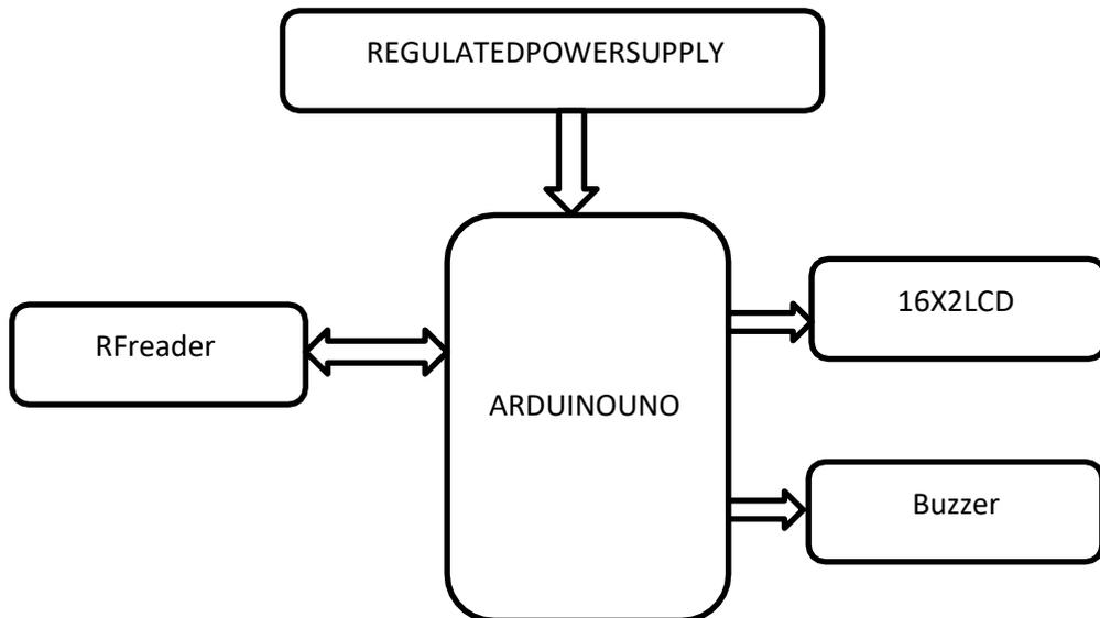
Fig 3.2: RFID to authenticate track data
