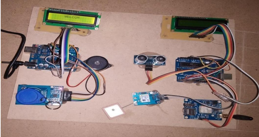
Fig6.1.3: Authorized key scanned to RFID Scanner
