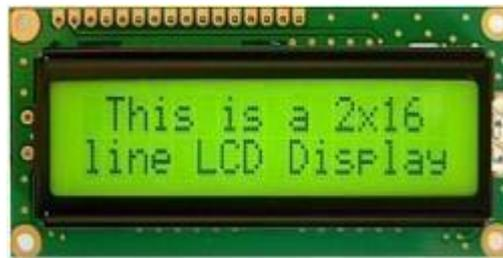
**Fig 3.5.1: 2x16 Line Alphanumeric LCD Display**
