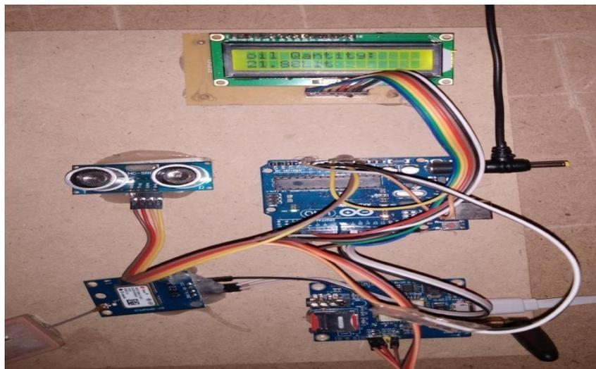
Fig6.2.1: LCD displays Quantity of oil in the truck
