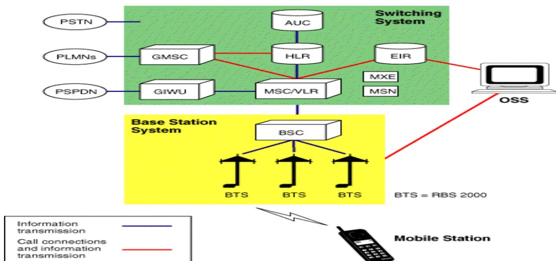
Fig3.3.5: Block diagram of GSM system
