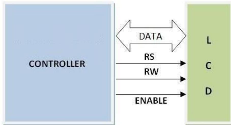
Fig 3.5.2: Interfacing with microcontroller
