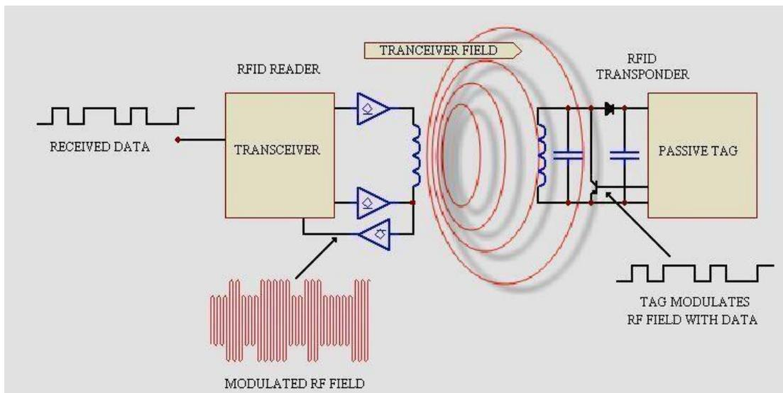
**Fig3.6.1: Working operation**
