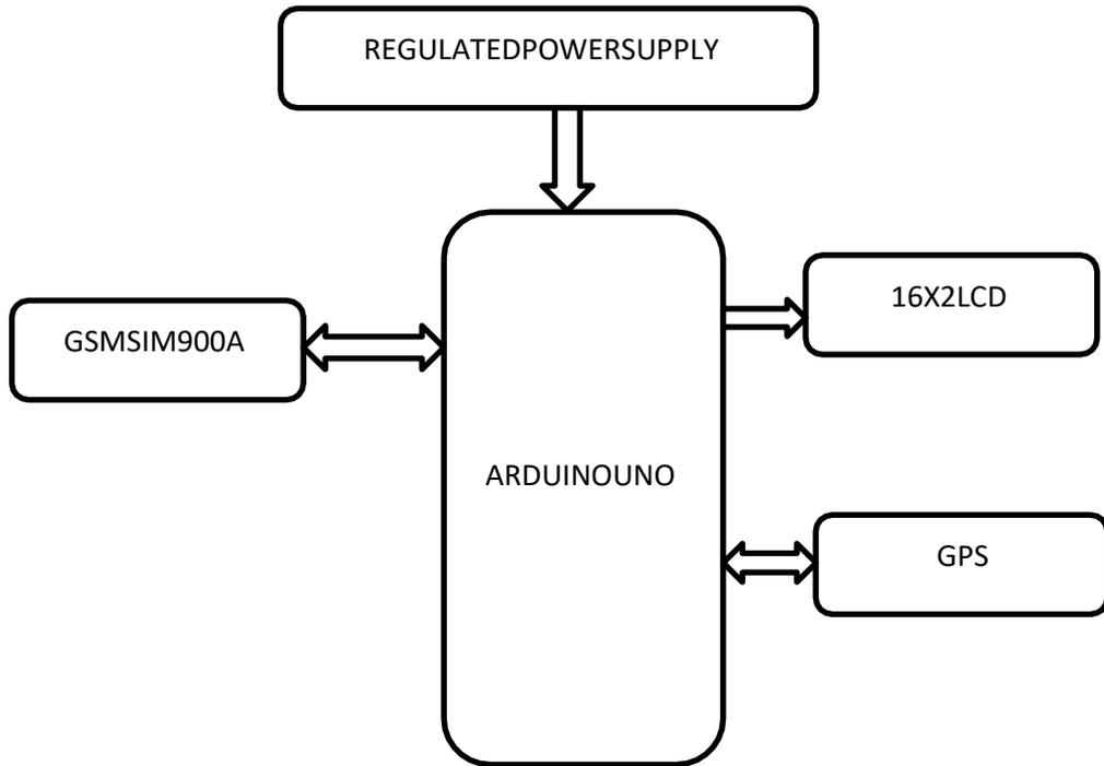
Fig 3.1: location tracking with GPS and GSM to send SMS
