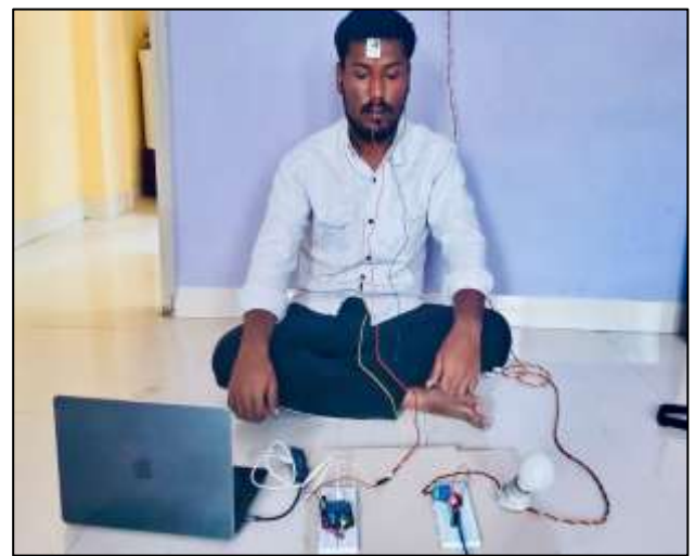
Fig -10: Experimental validation of the proposed Brain-Controlled Assistive Device: (a) Low concentration state with bulb OFF
