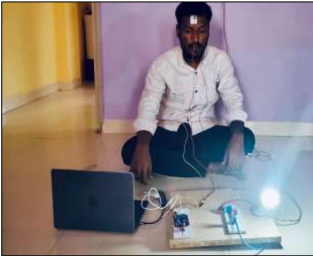
Fig -10: Experimental validation of the proposed Brain-Controlled Assistive Device: (b) High concentration state with bulb ON.
