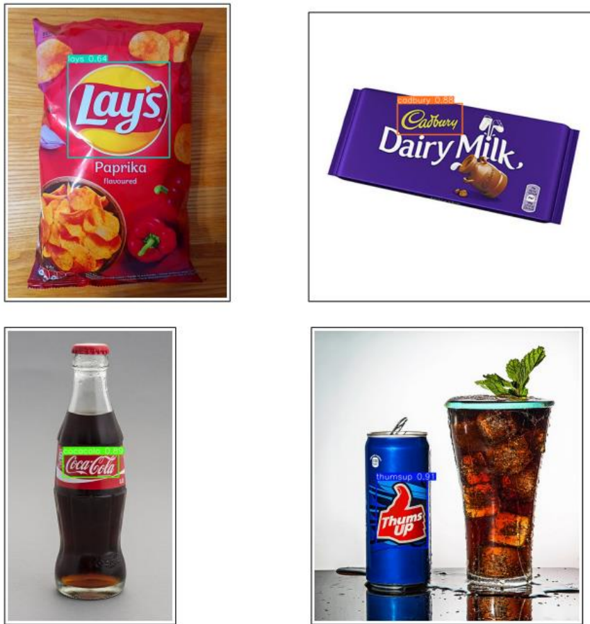
Figure 5: Results of detection of different logos using YOLOv5
