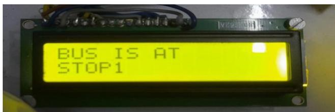
When the bus leaves the depot the driver turns on the first RF signal. This message is displayed on LCD. Then it checks SMS on his mobile and gets the location of the user. When the bus is near the desired location the bus driver turns on the second RF signal. This message is displayed on LCD.
