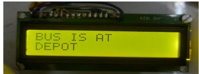
Upon the arrival of the bus, the announcement is made, the user boards the designated bus using obstacle detection and disables his location. When the bus leaves the depot It will send the first RF signal. The RF receiver in the user module receives this signal and turns on the buzzer. Then the user pushes a push button which sends the current location of the user to the bus driver.
