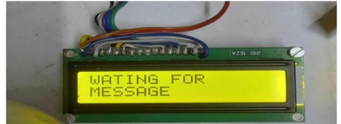
On triggering the bus module will send a RF signal to the bus station module. The bus station module on receipt of the RF signal makes an announcement about the bus and also displays the message on LCD. Meanwhile, the user module on receipt of the RF signal starts buzzing in a continuous manner.
