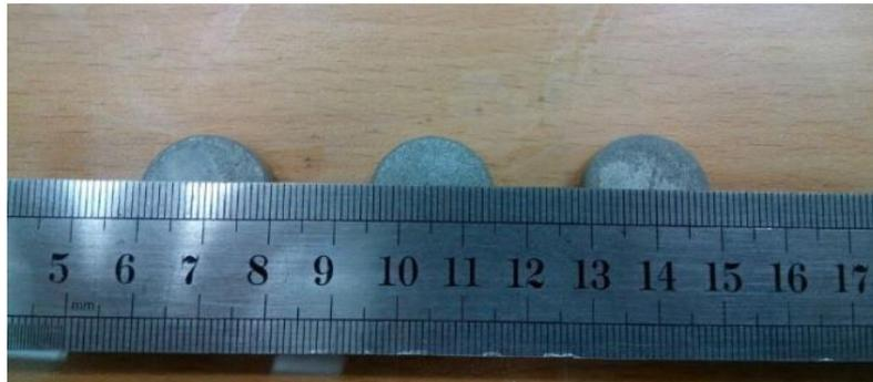
**Fig. 4.1: Showing prepared composites samples after sintering and Heat treatment.** It can be seen that only a slight variation in diameter is observed after sintering and the samples have diameters around 18-19 mm contrary to 20 mm initial diameter.
