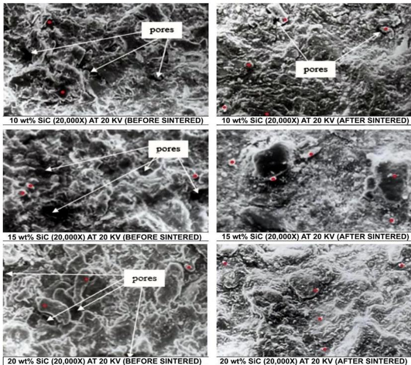
**Fig. 4.2: Showing SEM micrographs of Al-SiC reinforced MMCs. The SiC particles are highlighted with reddots to show their appearance.**
