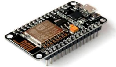
**Fig -9: Node MCU ESP8266**
