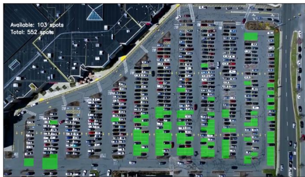
Fig. 11. depicts the empty car parking slots by using VGG16 CNN architecture
