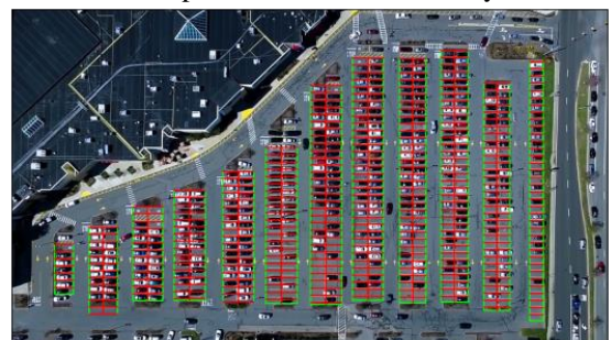
Fig. 6. Drawing rectangles at all the parking slots
