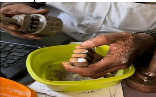
Creation – A manual compressor was used to create a small batch of coffee cubes, with an initial focus on structural stability and solubility.
