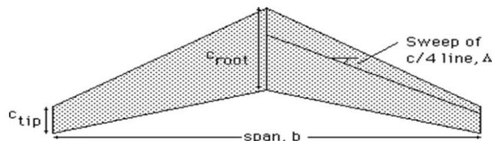
Fig 1: Wing Design Parameter
