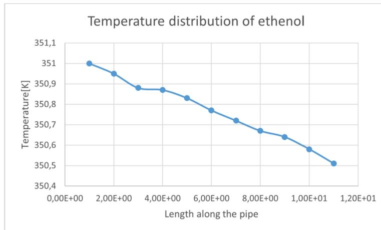
Temperature Distribution Graph for ethanoll in the triangular inner pipe.
