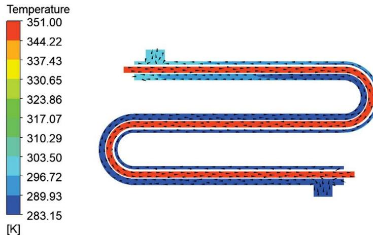
Temperature distribution in triangle- shaped inner pipe.
