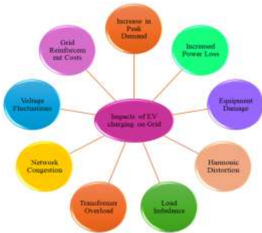
Fig.1. Various effects of EV charging on grid.
