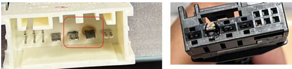
Picture 7: Reference and representative picture of harness side local melt and terminal blackening
