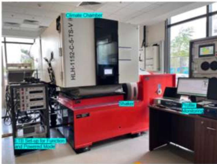
Picture 6: Reference and representative picture of the vibration test set-up
