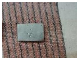
Fig 12- specimen undergone hardness testing
