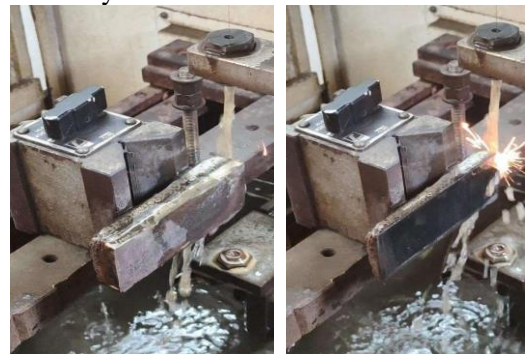
Fig 8- Wire EDM machine used for cutting specimen
