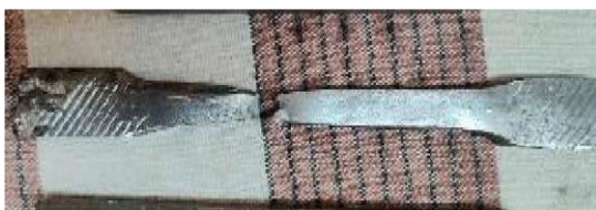
Fig 11- Specimen after tensile testing
