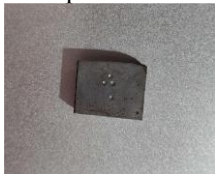
Fig 10- A small piece is cut for hardness testing
