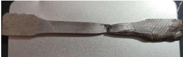
Fig 9- Specimen cut in the shape of dumbbell
