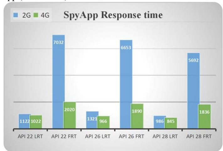
Fig 5.2(b): Response time comparison for SpyApp(parent’s side)
