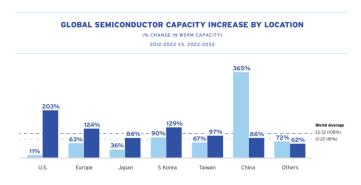
Fig. 3. Global Semiconductor Capacity Increase by location, WSPM(Wafer Starts Per Month), Source: 2024 state of the U.S. semiconductor industry [8]
