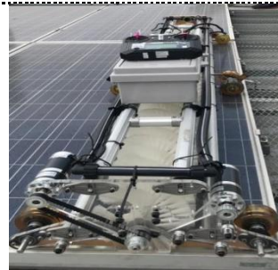
Figure 10. Robot for cleaning solar panels in laboratory environment with a length of (a) 2meters and (b) 4 meters.
