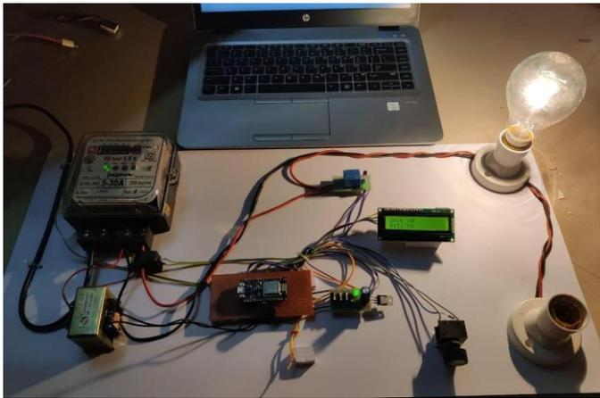
Fig 4.1 Hardware Of The Smart Energy Meter
