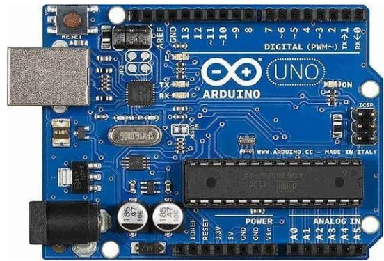
**1. Microcontroller Board :** Arduino Uno is an open-source microcontroller board based on the ATmega328P chip. It has 14 digital input/output pins, 6 analog inputs, and operates at 5V.
