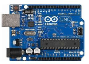
**1.Microcontroller Board** : Arduino Uno is an opensource microcontroller board based on the ATmega328P chip. It has 14 digital input/output pins, 6 analog inputs, and operates at 5V.
