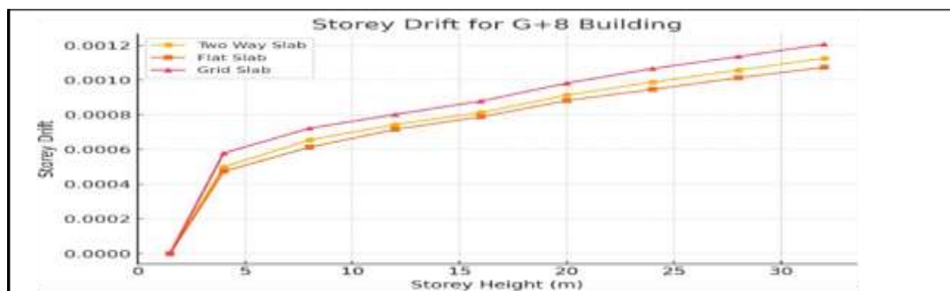
Figure 11: Storey Drift for G+8 Building
