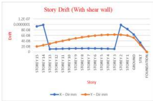
Fig. 5.4: Storey drift chart (With shear wall)
