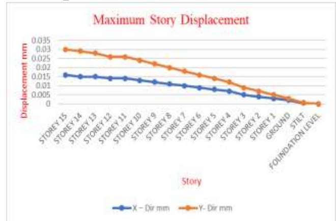
Fig. 5.1: Storey displacement chart (Without shear wall)
