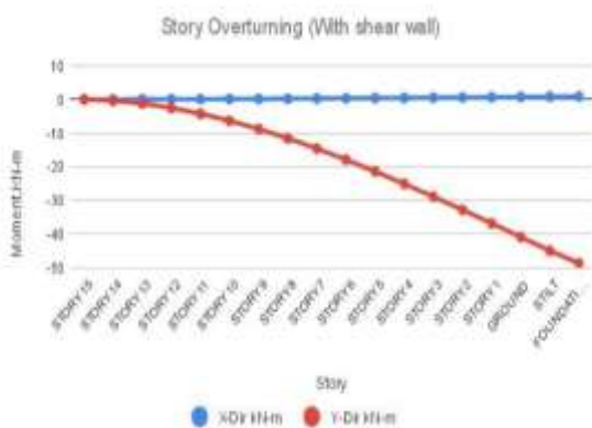
Fig. 5.6: Storey overturning chart (With shear wall)
