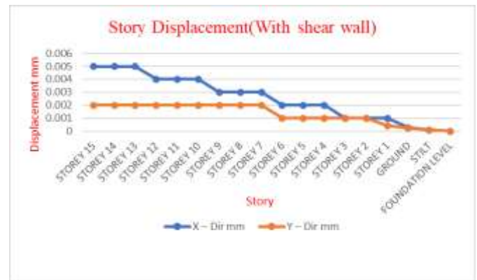
Fig. 5.2: Storey displacement chart (With shear wall)
