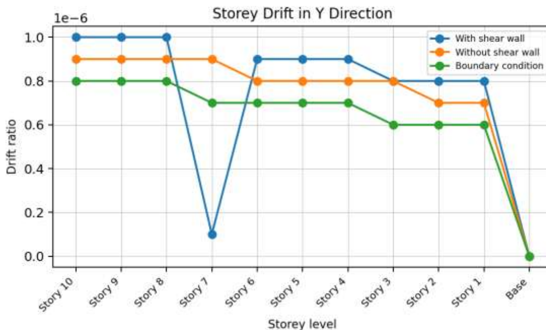
Figure 4. Storey drift profile in Y direction
