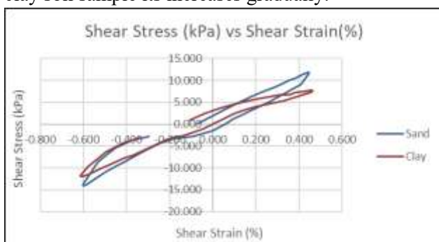
Figure 5-Stress Strain Hysteric loop response for 30 th cycle (amplitude+0.1)
