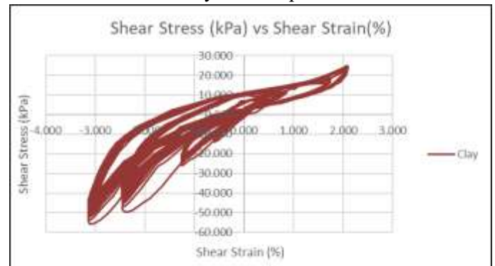
Figure 3- Stress Strain hysteric loop response of Clay
