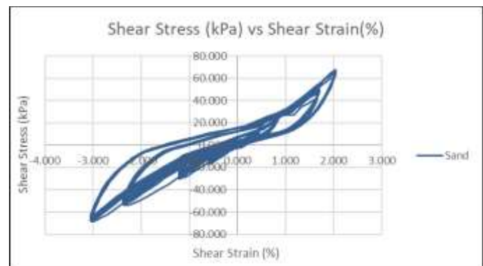
Figure 4-Stress Strain hysteric loop response of Silty Sand
