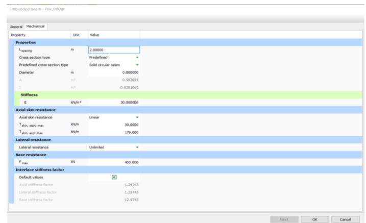
Figure 5: Plaxis 2D input for Pile Modelling
