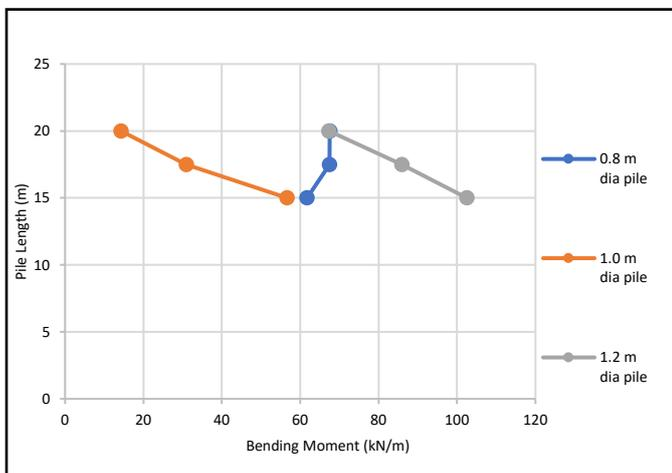
**Figure 14: Graph for Bending Moment Vs Pile Length by keeping pile spacing constant**
