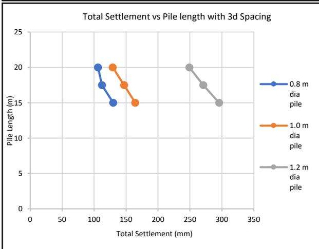
**Figure 11: Graph for Total Settlement Vs Pile Length by keeping pile spacing constant**
