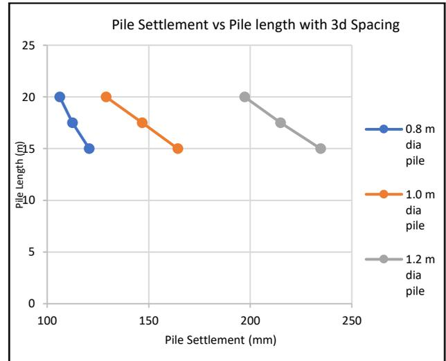
**Figure 12: Graph for Pile Settlement Vs Pile Length by keeping pile spacing constant**
