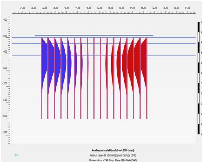
Figure 10: Bending moment in piles
