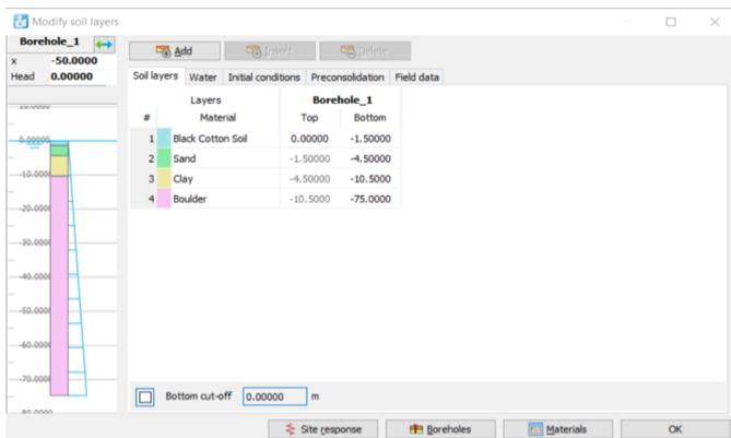
Figure 3: Plaxis 2D input for Soil layers
