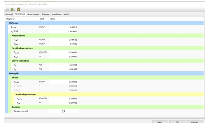
Figure 4.: Plaxis 2D input for Geotechnical Parameters
