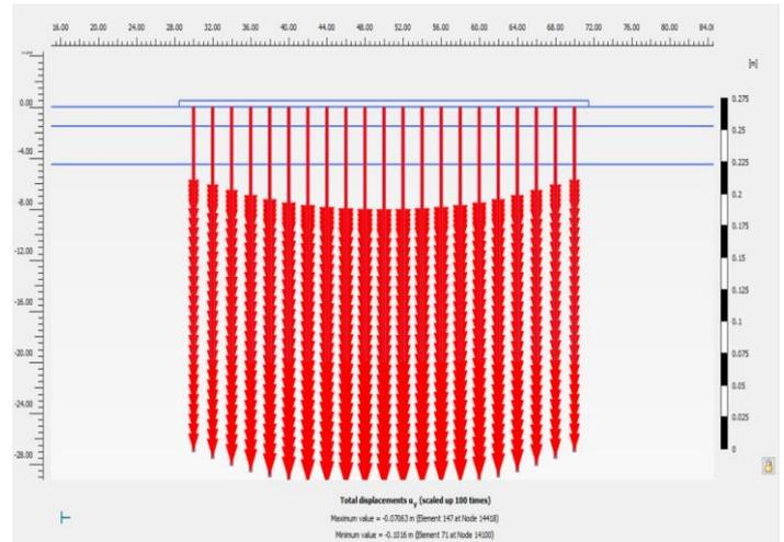
Figure 8: Pile settlement at the base of pile cap
