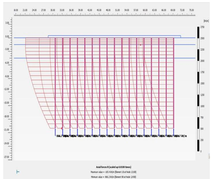
Figure 9: Axial force in piles
