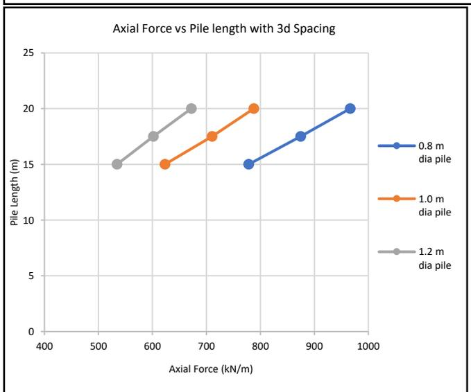
**Figure 13: Graph for Axial Force Vs Pile Length by keeping pile spacing constant**
