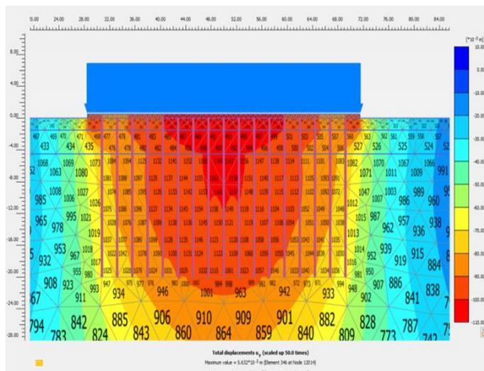
Figure 7: Settlement under pile cap
