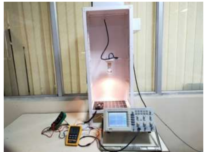
Fig -5: Indoor set up with Loom 10 Wp Polycrystalline solar panel for Hardware verification
