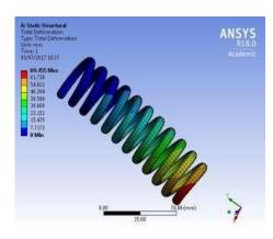
Fig -7: Maximum deflection contour of composite helicalspring at 1281.7 N
