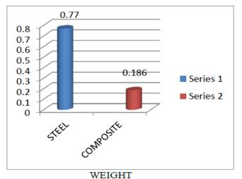
Fig -9: Comparison graph result of weights in steel HelicalSpring and composite helical spring.
