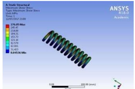
Fig -6: Maximum shear stress contour of composite helical spring at 1281.7 N
