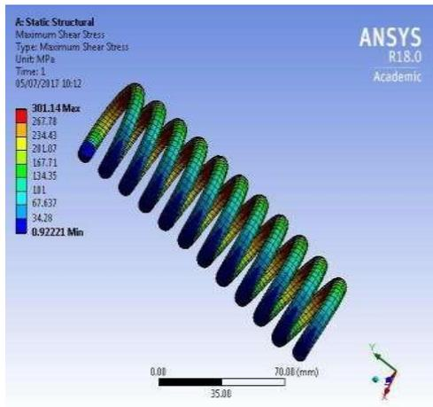
Fig -4: Maximum shear stress contour of steel helical spring at 1281.7 N.
