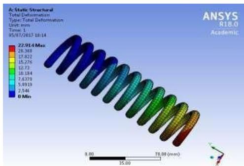
Fig -5: Maximum deflection contour of steel helical spring at 1281.7 N.
