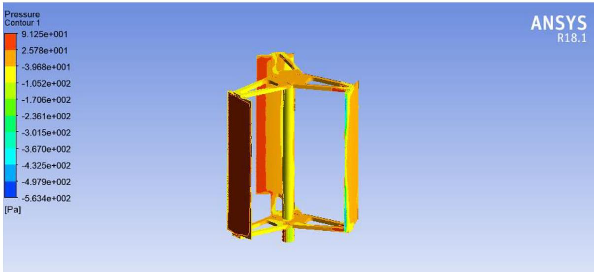
**Figure 11:- Pressure Contours**
