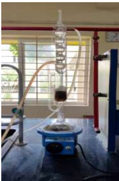
Fig-1: Soxhlet extraction of clove buds with ethanol
