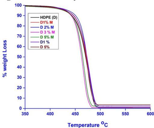
Figure 2: TGA analysis for waste HDPE (B) and HDPE/clay nanocomposites.
