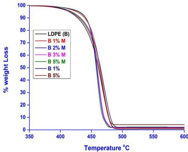
Figure 1: TGA analysis for waste LDPE (B) and LDPE/clay nanocomposites.
