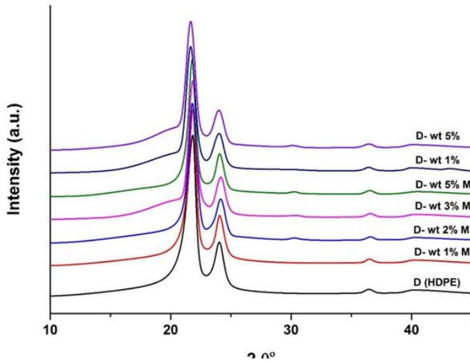
Figure 3: X-ray diffraction curves of waste HDPE, Chemical container (D) and waste HDPE /clay nanocomposites, where M is mean the modified clay.
