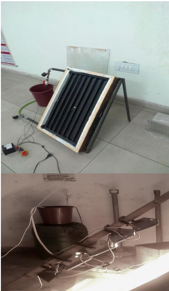
Figure Flat plate solar collector
