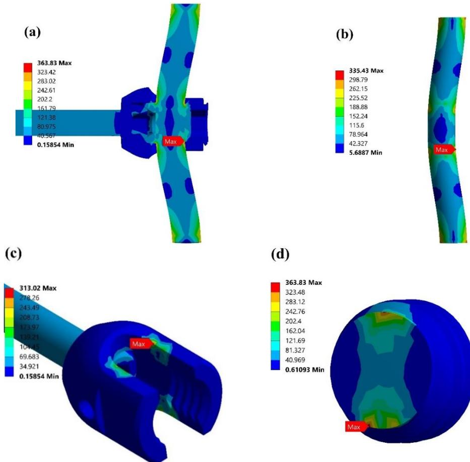
Fig -7: Trend of Tresca stresses in (a) Pedicle subassembly, (b) Rod, (c) Screw and (d) Tightening screw during Anterior-Posterior test.
