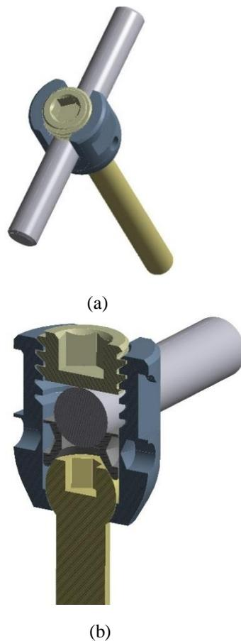
**Fig -4:** CAD-model of (a) Pedicle screw, (b) Cross-section view of the pedicle screw
