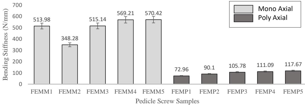
Fig -6: Bending stiffness of mono axial and poly axial screws obtained for FE moment Test
