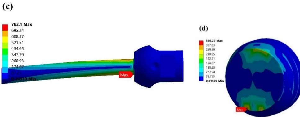
Fig -9: The trend of tresca stresses in (a) Implant assembly, (b) Rod, (c) Screw and (d) Tightening screw during the Flexion-Extension moment test.
