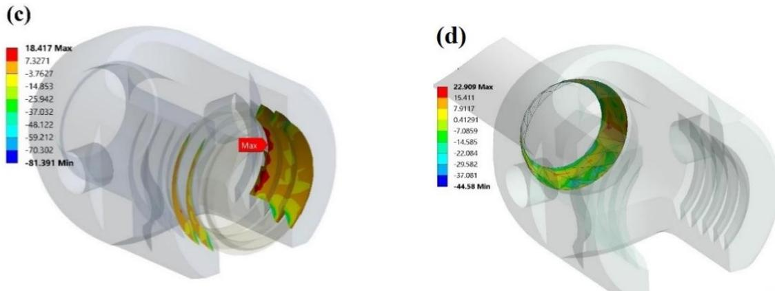
**Fig -8:** Contact Pressure distribution acting at the contact between (a) Rod and tightening screw, (b) Fixation rod and cap, (c) Threads of tightening screw and screw head (d) Screw and screw head during Anterior-Posterior test.
