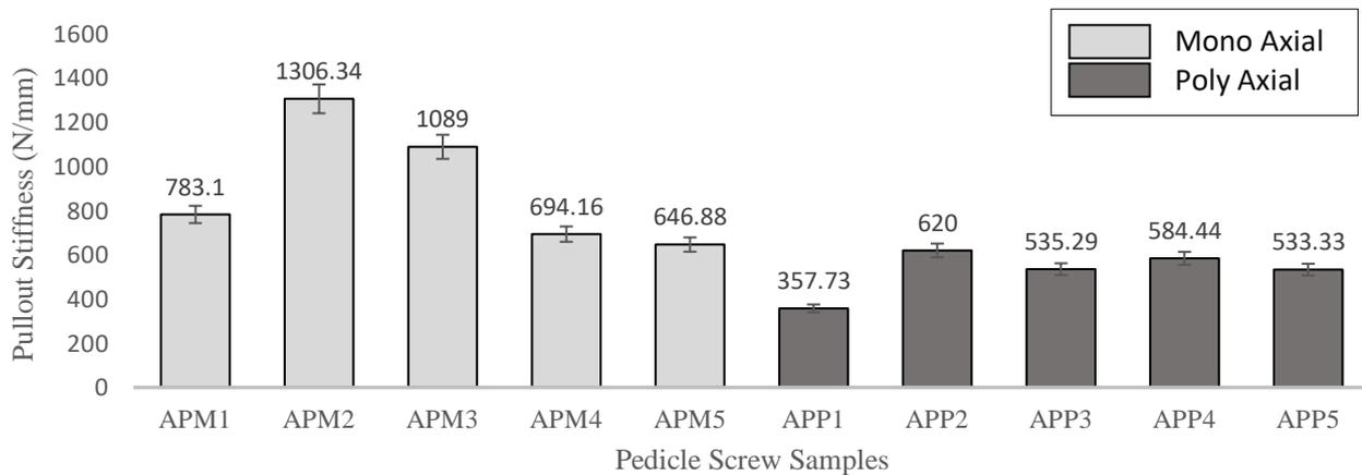
**Fig -5:** Pullout stiffness of Mono axial and Polyaxial screws obtained for AP Test
