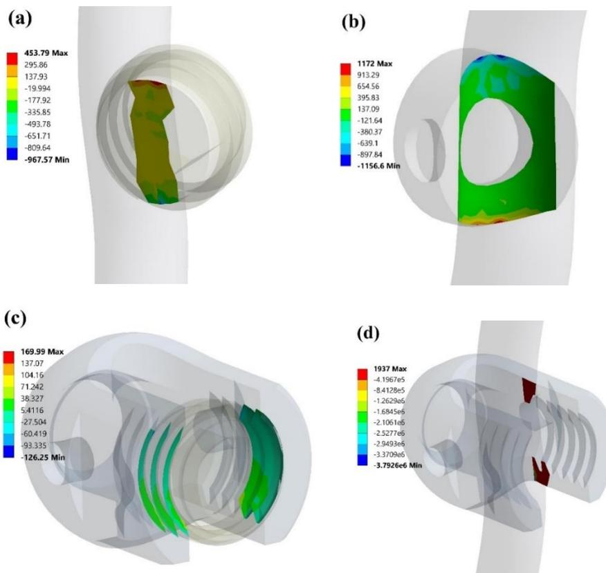
Fig -10: Contact Pressure distribution acting at the contact between (a) Rod and tightening screw, (b) Fixation rod and cap, (c) Threads of tightening screw and screw head (d) Rod and screw head during Flexion-Extension Test.
