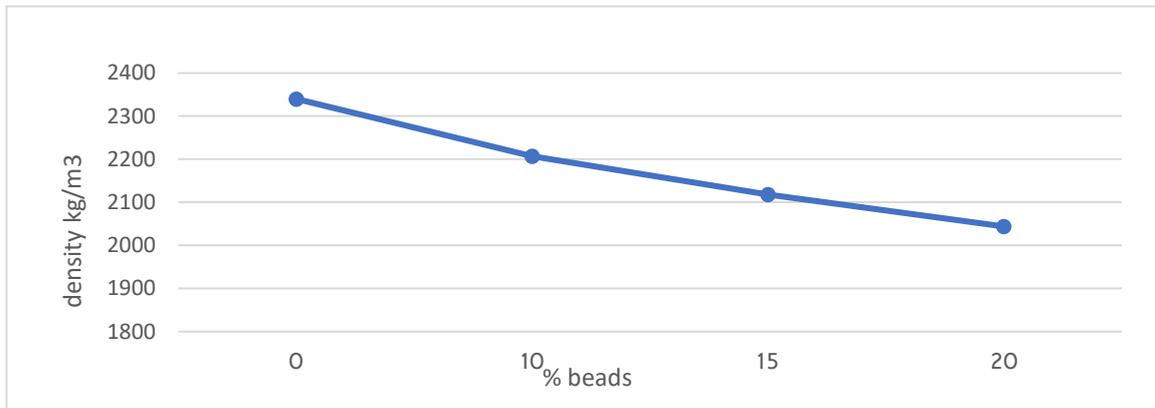
The study identifies the maximum and minimum densities as 2340 kg/m<sup>3</sup> and 2044 kg/m<sup>3</sup>, respectively, corresponding to 0% and 20% aggregate replacement with beads. The density and the percentage of beads, which lowers the weight of the concrete, are directly correlated in this figure.
