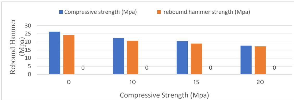
In the data shown in the graph, a comparison between destructive and non-destructive tests for strength is made using only the compression test and rebound hammer test, not the ultrasonic pulse velocity test. This is because the ultrasonic test only shows the homogeneity and quality of concrete, not its strength. The strength obtained from the destructive test is comparatively higher than the strength measured by the rebound hammer test.
