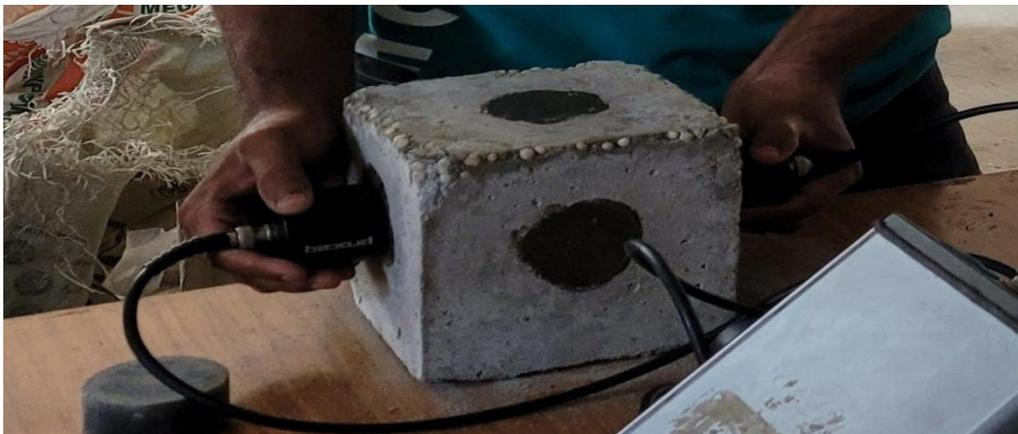
Ultrasonic pulse velocity test
