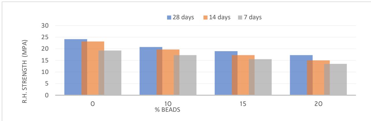
(a).7 Days Test Of Compressive Vs Rebound Hammer Strength (Mpa)
