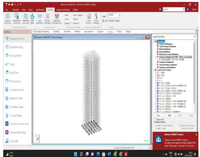
Fig.5 (a) Assigning Load case and Definitions
