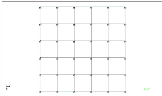
Fig.3 (a) Assignment of Fixed support
