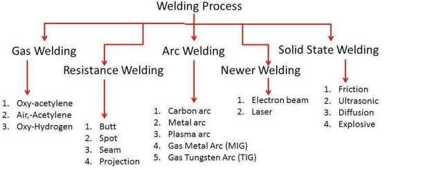
**Arc Welding**: Arc welding is a type of fusion welding that uses a welding power supply to create an electric arc between an electrode and the base material to melt the metals at the welding point. They can use either direct (DC) or alternating (AC) current, and consumable or non-consumable electrodes. Two major types of arc welding are MIG and TIG welding.
