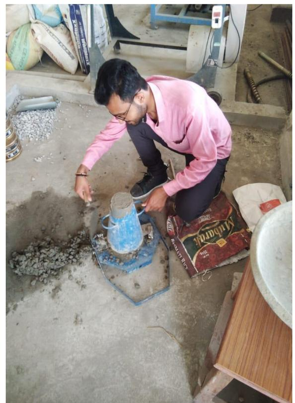
Figure 1: Slump Test
