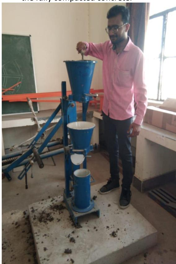
Figure 2: Compaction Factor Test
