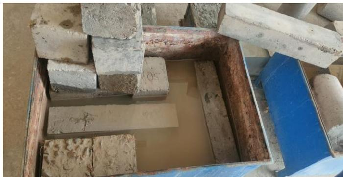
Figure 3: Test specimens being cured in curing tank
