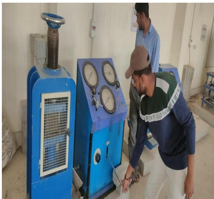
Figure 4: Compressive Strength Test
