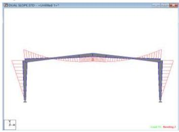
• Shear forces in mono-slope columns were higher compared to dual-slope sheds.
