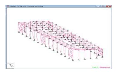
• Dual-slope shed exhibited lower and more uniform deflection due to symmetric load distribution.
