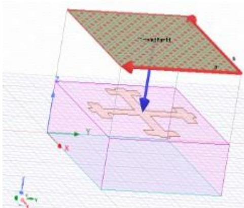
Fig. 2.b. Metamaterial-based Jerusalem cross-patch antenna
