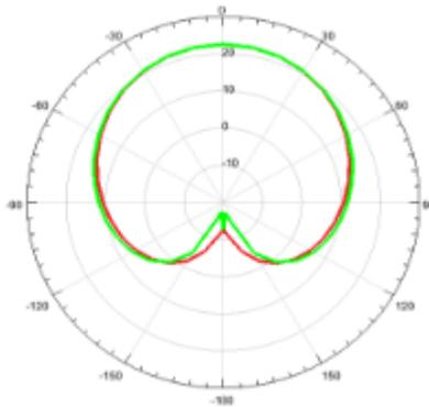
Fig. 3.c. Gain plot for jerusalem cross patch antenna
