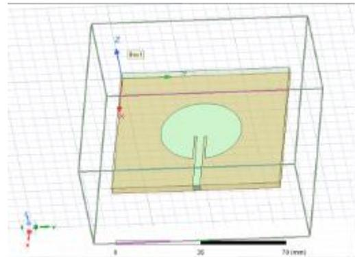
Fig. 2.a. Circular Patch Antenna
