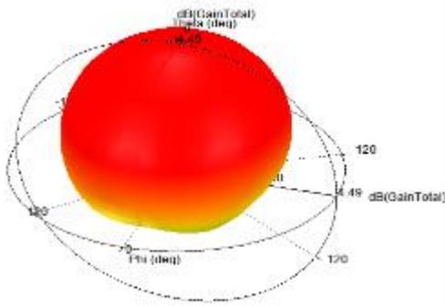
Fig. 3.b. 3D polar plot for circular microstrip patch antenna
