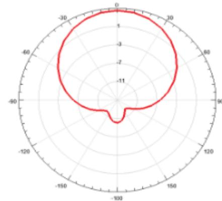
Fig. 3.a. Gain plot for circular microstrip patch antenna
