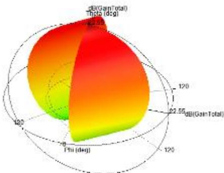
Fig. 3.d. 3D polar plot for jerusalem cross patch antenna
