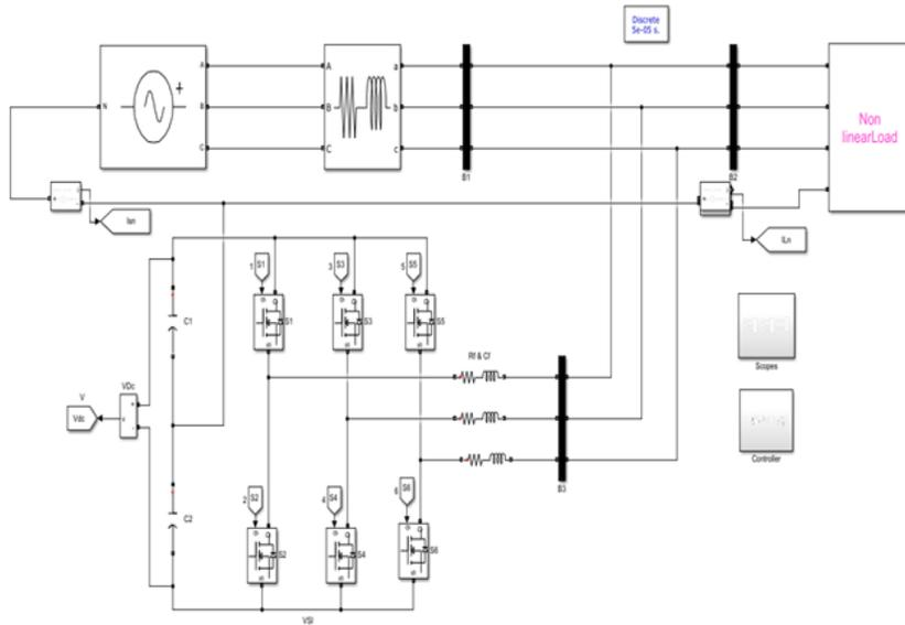
**Fig 1 Simulink Model of Controlling System**
