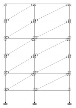
Fig.1: An Infill Building without soft storey
