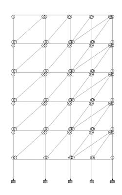
Fig.2: Modelling of infill walls (front view)
