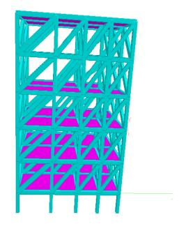
Fig.3: Modelling of infill walls (side view)
