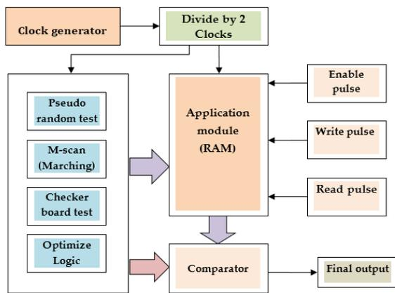
Fig. 1. shows the system architecture developed in VHDL configurable logical blocks using behavioural modelling in FPGA.
