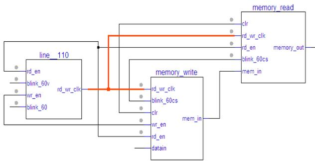
Fig 6. Internal architecture Memory BIST
