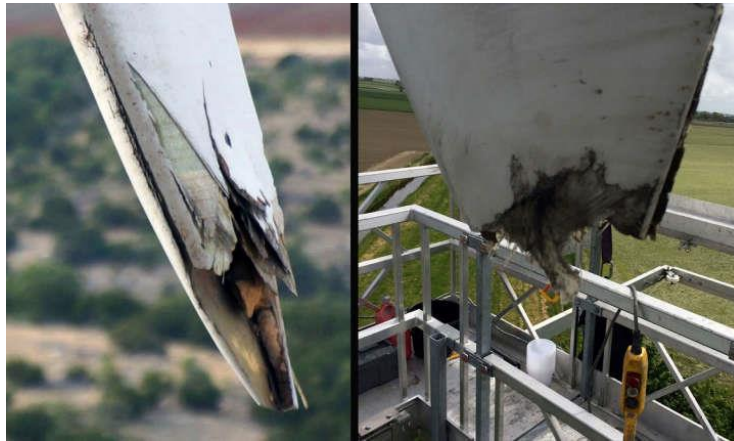
Figure 2: Damaged Turbine Wind Blade due to lightning
