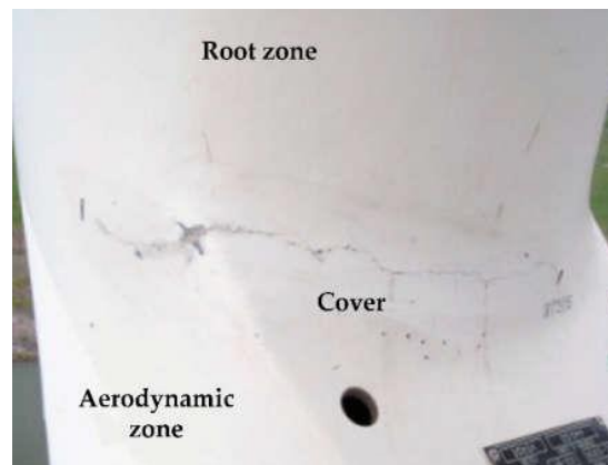
Figure 3: Damaged Turbine Wind Blade due to Fatigue
