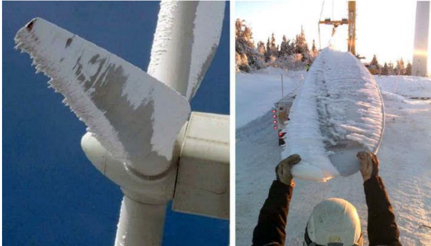
Figure5: Damaged Turbine Wind Blade due to Icing
