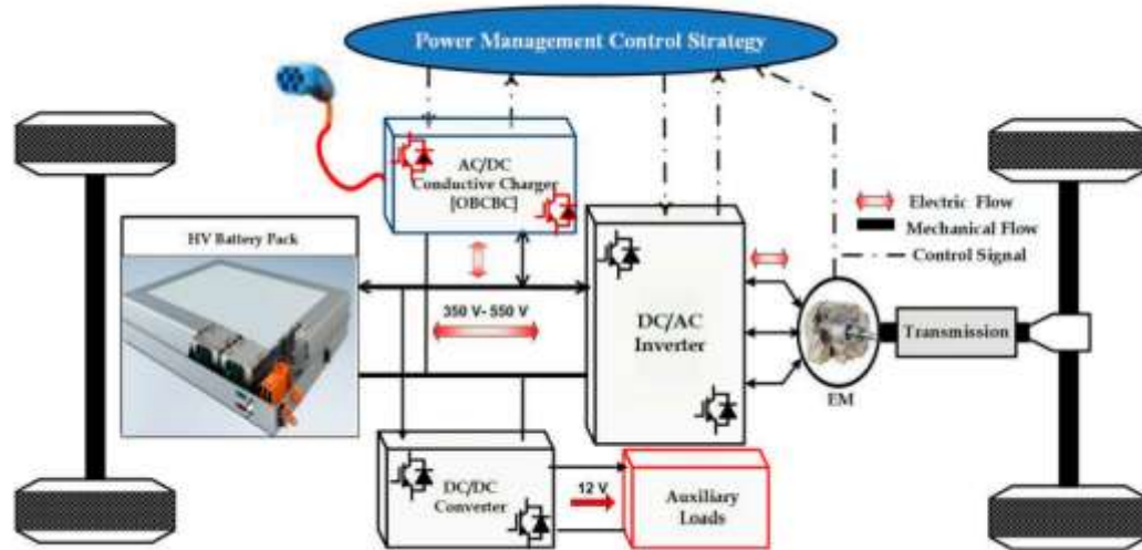
Fig 1. Electric vehicle's components.
