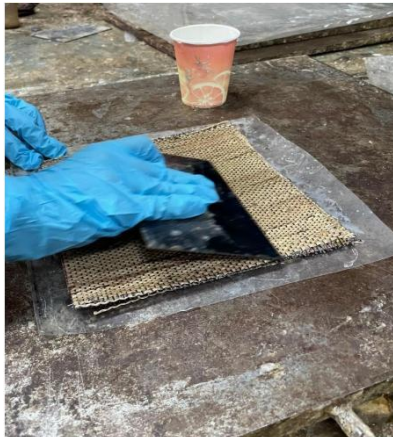
Figure 33: Hand Lay Up of Areca Nut/Epoxy Composite Laminate
